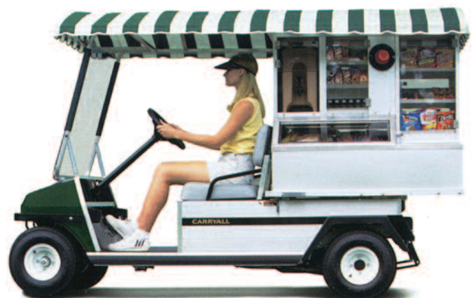
Model PC-LC-480-BC-CC Powered by 11 hp, 351 cc, gas, air-cooled engine.
